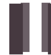
Scorrevole esterno muro 2 ante sovrapposte doppie Outside the wall sliding door with two overlapping double leaves
