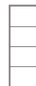
cieca 4 riquadri e 3 profili in alluminio satinato blank with 4 sections and 3 satin aluminium profiles
