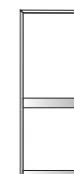
cieca con fascia centrale paracolpi e zoccolo in alluminio satinato flush with satin-finish aluminium strip and kick plate
