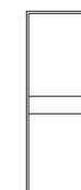
cieca con riquadro centrale e 2 profili in alluminio satinato blank with central section and 2 satin aluminium profiles
