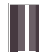
Scorrevole interno muro 2 ante sovrapposte doppie Inside the wall sliding door with two overlapping double leaves
